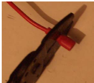
Where to Crimp the Spade Terminals
