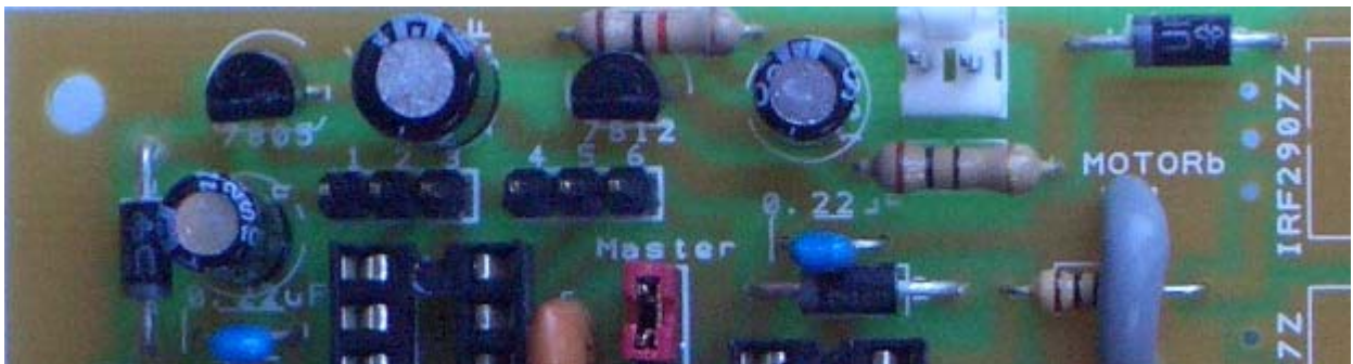
Power Regulation Section on PCB
