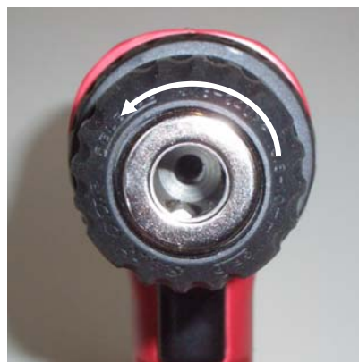
To Remove the Chuck Twist it Anticlockwise
