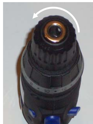
To Remove the Chuck Twist it Anticlockwise
