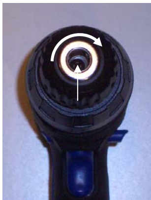
To Remove the Chuck Screw Twist the Screw Clockwise
