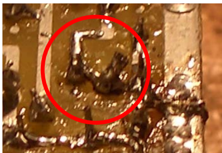
A Solder Bridge Between Two Tracks Causing A Short
