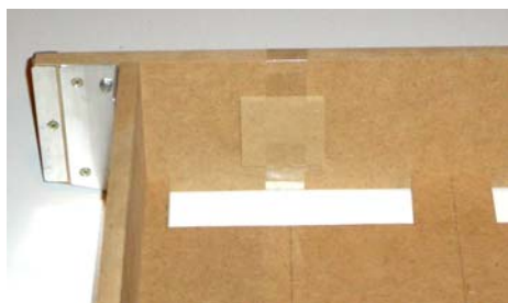
6mm MDF Used As a Temporary Spacer
