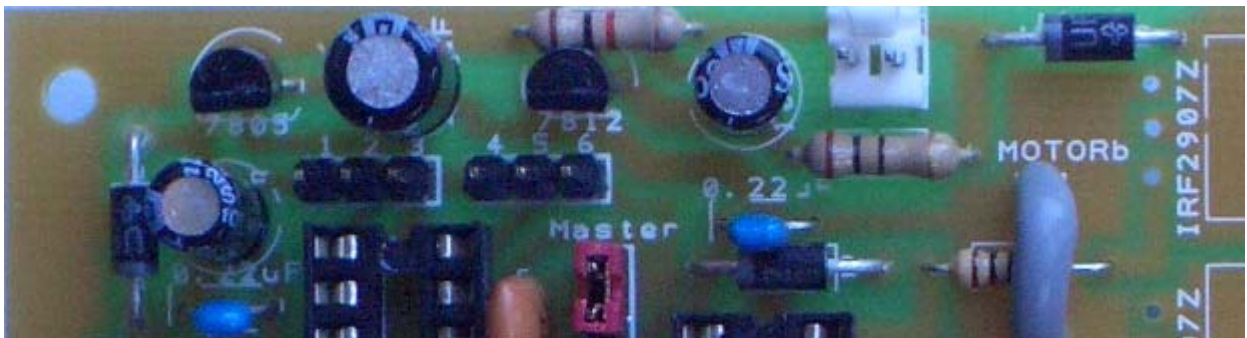
Power Regulation Section on PCB
