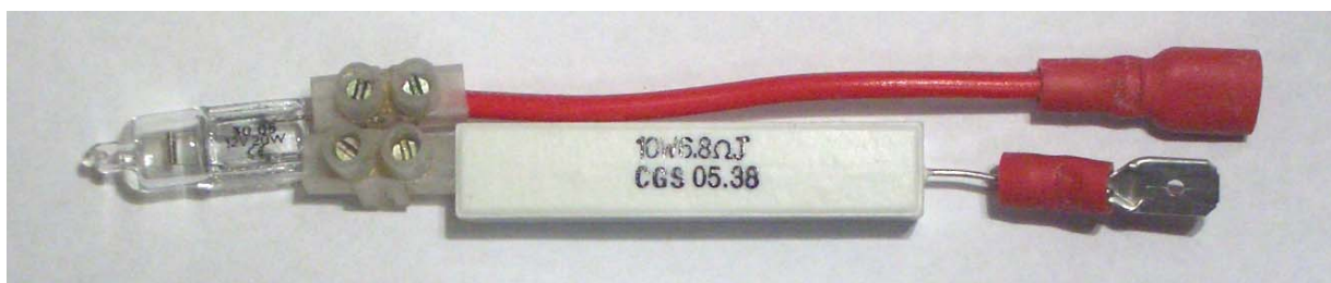
12v Halogen Bulb and 6R8 10W Resistor For Initial Testing of Small Motor
