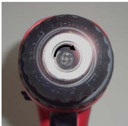
To Remove the Chuck Screw Twist the Screw Clockwise
